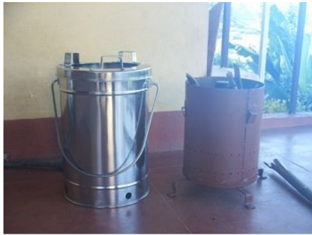
Fig 9: The two major parts of the Sampada stove
