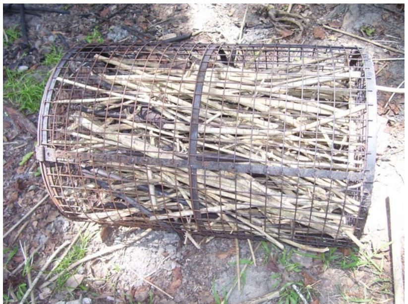
Fig 36: Wire mesh cage for holding feedstock, this makes it easier to load and unload the drum
