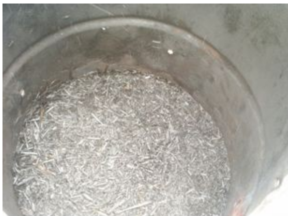
Fig 29: Wood shavings inside the single barrel reactor
