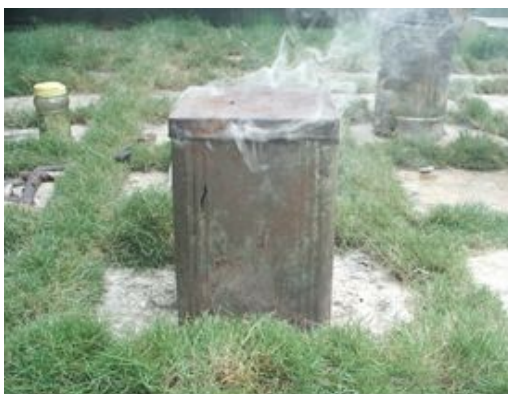
Fig 15: Airtight can aiding in the charring process
