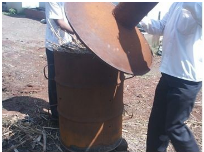
Fig 28: Filling the barrel with biomass
