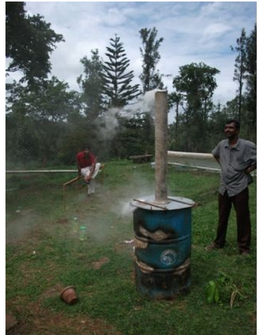
Fig 24: Double barrel pyrolytic reactor in operation
