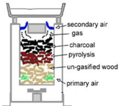
Fig 11: Working of the Sampada Stove
