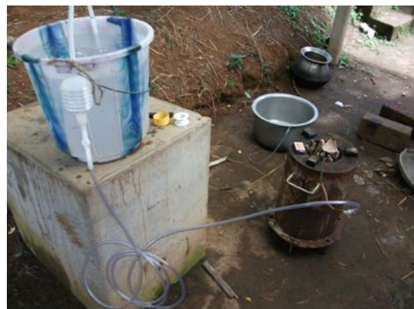
Fig 8: Photograph of the copper coil water heating set up
