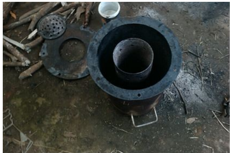
Fig 2: Upside down Anila stove, for loading biomass to be charred
