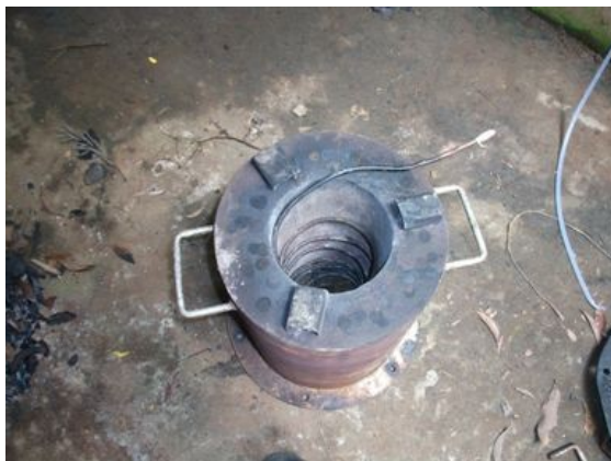
Fig 7: Copper coil inserted inside the combustion chamber of the Anila stove
